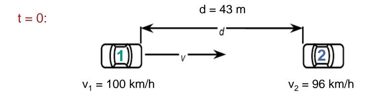
Until now the simulation determines the distance between the vehicles and the difference in the relative speed. In the next step the velocity of car 1 should be controlled so that the distance between the cars stays constant. That means that the velocity of car 1 should be lowered to the speed of car 2.
