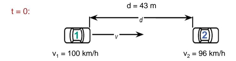
In the following simulation two cars drive behind one another with a certain velocity and a fixed distance at the beginning (t=0). Due to the difference in velocity the distance between the cars will change over the simulation duration. The situation is seen form the view of a radar in car 1 (ego car), the vehicle ahead car 2 represents the radar target.
